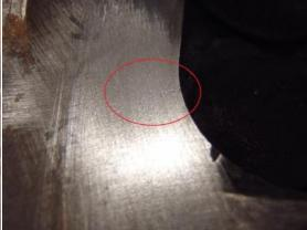
The cylinder head should be checked for a broken back. This is a long crack running (picture right) between core plugs. This condition is quite uncommon, and is suspected to relate to rocker shaft removal without slacking remaining head bolts. An engine with coolant leaking into in the oil is a good clue of this condition.
