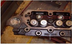
Even if your cylinder head was "working perfectly" with a crack, its presence has weakened it, and as a policy we do not sell or remanufacture heads with these defects.
